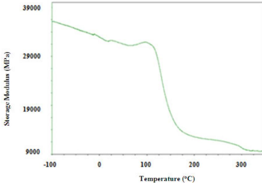
Figure 12 Flexural modulus of elasticity of GFRP bar specimen found by DMA between  $-100^{\circ}$  and  $350^{\circ}\text{C}$
