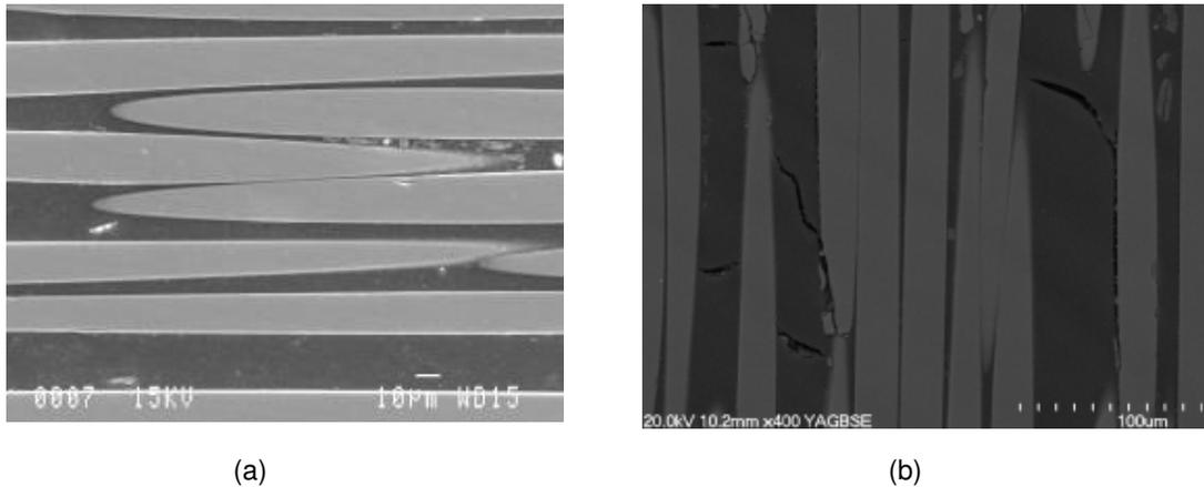
Figure 15 Micrographs of longitudinal fibre/ matrix interface of: a) unconditioned GFRP bar specimen, b) Conditioned GFRP bar specimen aged in air at 350°C for 2 hours.
