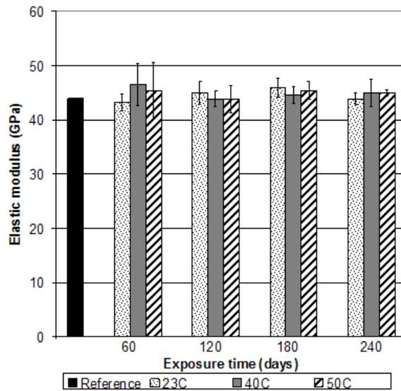
Figure 6 Elastic modulus retention of conditioned GFRP bars aged in moist concrete at 23°, 40°, and 50°C
