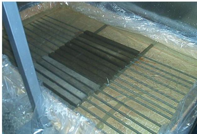
Figure 3 Wood container built for aging of the cement mortar-wrapped GFRP bar specimens
