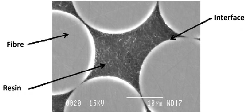
Figure 2 Typical microstructure of GFRP bar
