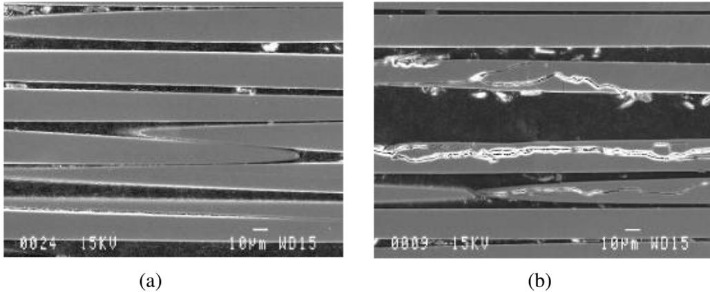
Figure 8 Micrograph of longitudinal GFRP bar surface pre-loaded under tensile load: a) Reference GFRP bar at low magnification, and b) GFRP bar loaded at 80% of the UTS at high magnification
