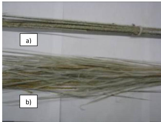
Figure 13 The failure mode of GFRP bars : a) tested at room temperature, and b) tested at  $150^{\circ}\text{C}$ .
