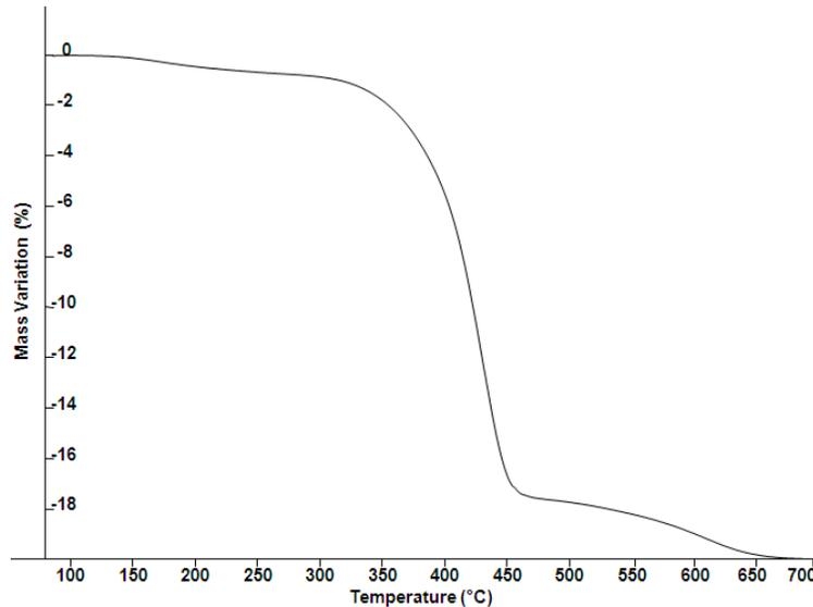
Figure 14 Mass variation of GFRP bar specimen when heated between 20° and 800°C.
