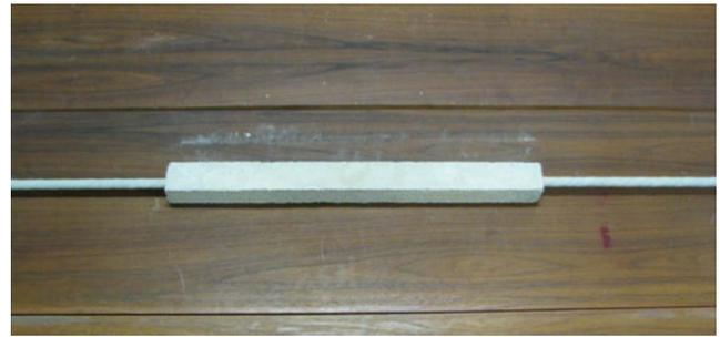
Fig. 2. View of cement mortar-wrapped GFRP bar specimen
