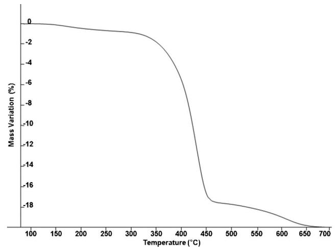
**Fig. 10.** Mass variation of GFRP bar specimen when heated between  $20^{\circ}$  and  $800^{\circ}$  C
