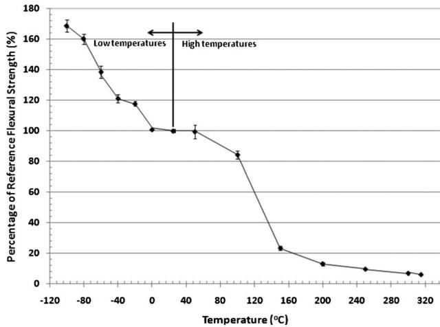
**Fig. 5.** Average flexural strength with standard deviation of GFRP bar specimens tested under different temperatures
