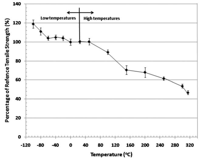
Fig. 3. Normalized average tensile strength with standard deviation of GFRP bar specimens tested under different temperatures
