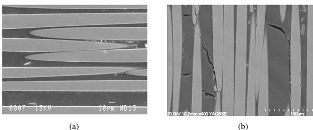
**Fig. 11.** Micrographs of longitudinal fiber/matrix interface
