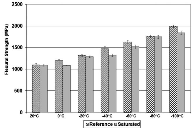
**Fig. 9.** Average flexural strength and standard deviation of unconditioned and saturated GFRP bars tested at low temperature
