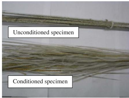
**Fig. 7.** Failure mode of unconditioned and conditioned specimens after tensile tests
