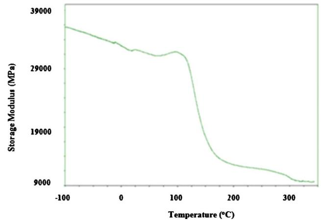
**Fig. 6.** Flexural modulus of elasticity of GFRP bar specimen found by DMA between  $-100^{\circ}\text{C}$  and  $350^{\circ}\text{C}$
