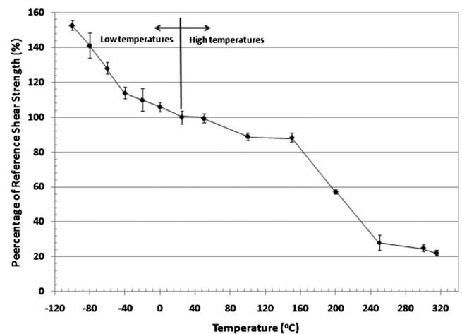
Fig. 4. Normalized average shear strength with standard deviation of GFRP bar specimens tested under different temperatures
