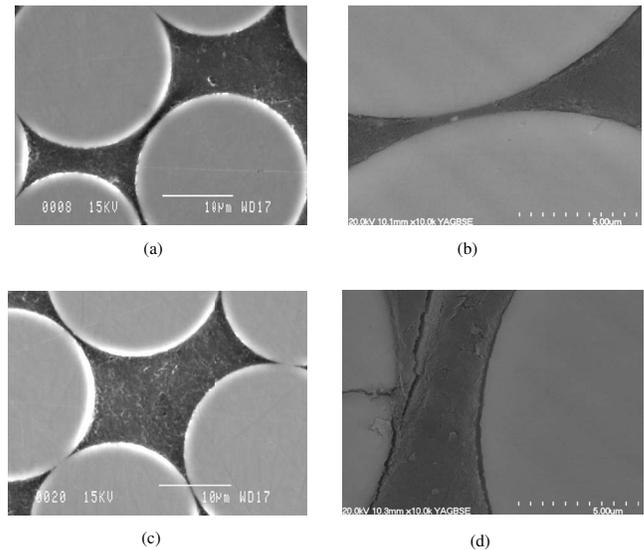
**Fig. 12.** Micrographs of transversal fiber/matrix interface
