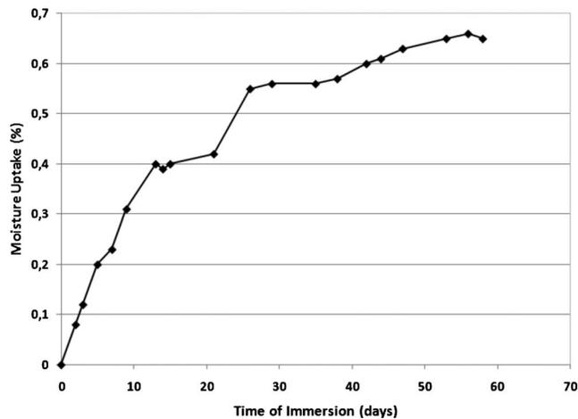
Fig. 1. Moisture absorption curve for 12.7-mm GFRP bar
