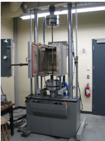
Fig. 2. Tensile test specimen in environmental chamber
