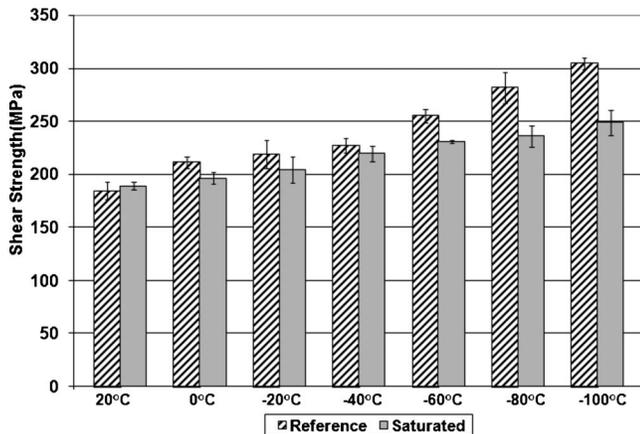
**Fig. 8.** Average shear strength with standard deviation of unconditioned and saturated GFRP bars tested at low temperature
